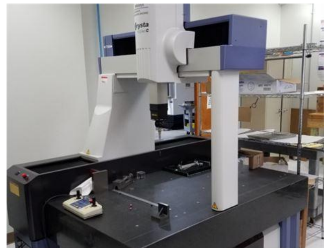
Figure 14. Checking on the coordinate measuring machine.
