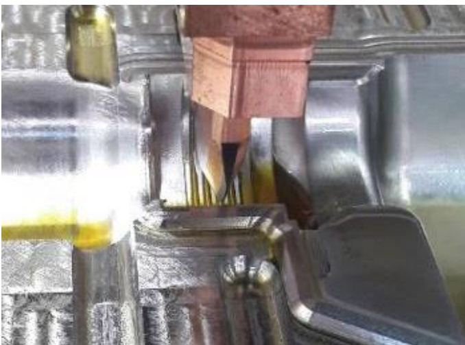
Figure 12. Electrical erosion machining of the threaded area.
